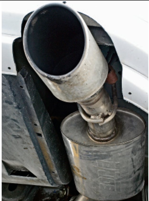
> Borla's '05-'06 GTO exhaust system is a true dual-pipe system all the way back to the rear bumper. Installing the right-side pipe on an '04 requires cutting a clearance slice out of the bumper, as shown here.
