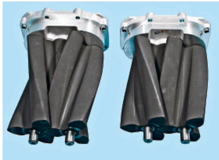
> With their high-helix rotors, Magnuson/Eaton superchargers are more efficient than old-school GMC Roots blowers. The longer Magnuson 122 rotors (left) have about 9 percent more capacity than the 112 rotors (right).
