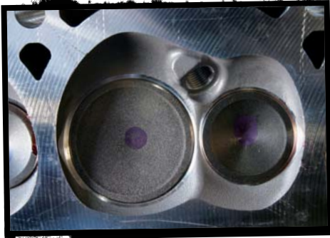
The intake valve is a massive 2.165 inches in diameter, while the exhaust is relatively tame at 1.59 inches. The combustion chamber measures 70 cc.
