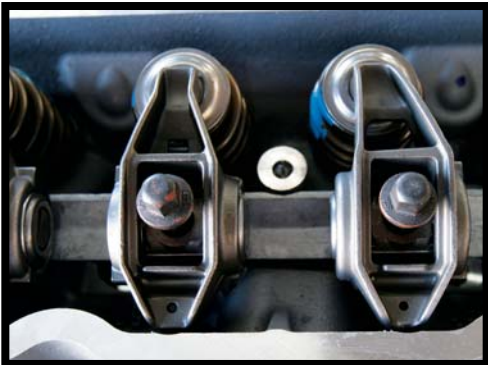
The wider, rectangular intake port moves the pushrod laterally, which requires an offset intake rocker arm. This is the first situation we can recall where a GM production engine uses an offset rocker arm to clear a wide intake port.
