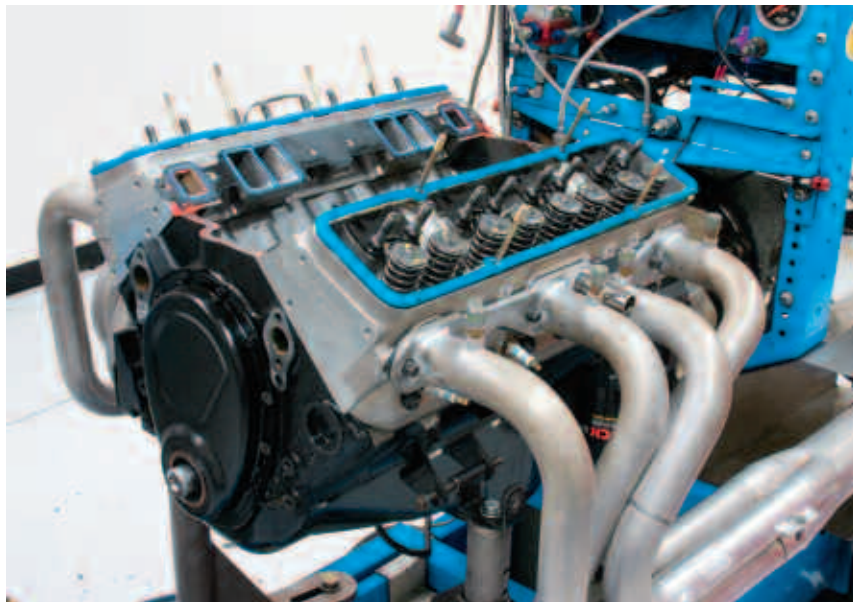
Our Fast Burn aluminum heads not only weigh nearly half that of an iron heads, but they made 44 hp and 27 lb-ft of torque more out of the box than a stock head.
