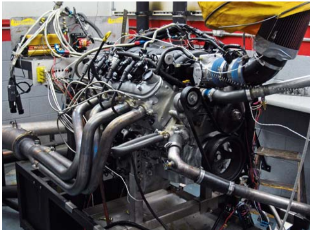
The assembled LS2 engine with the L92 heads and L76 intake looks very stealthy. In this form, the LS2 produced 546.8 hp at 6,500 rpm and 494.9 lb-ft of torque at 5,000 rpm. The short runners of the L76 intake and the good low-lift numbers of the L92 heads created an outstanding torque curve. This would be the hot setup for your typical full-weight street car.
