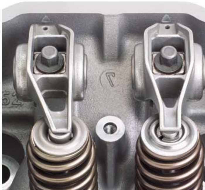
In order to make room for the wider rectangle intake port and larger valve sizes, it was necessary to use 6mm offset rocker arms on the intake side. The exhaust rocker arms remain unchanged from the LS2. This rocker configuration is also used on the 7.0L LS7.
