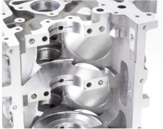
An internal view of the crankcase shows newly revised areas that have been reinforced and machined in order to increase structural strength of the bulkheads.
