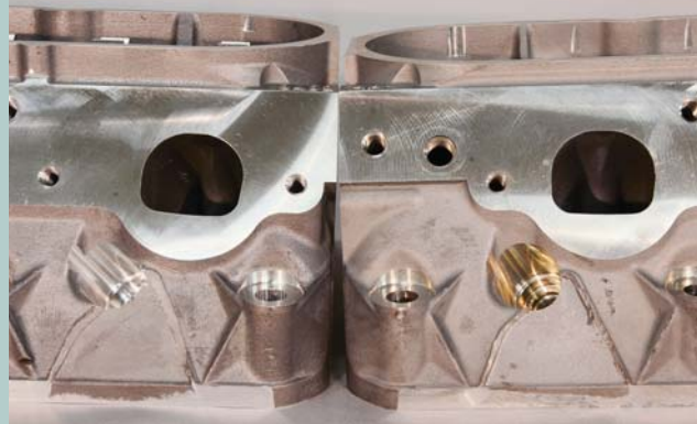
The exhaust ports of the LS7 and L92 are also quite similar, both using a D-shaped opening. In comparison to other Gen III and IV castings, says GM's Dennis Gerdeman, the L92 port opening is larger and the roof sits higher—so you'll need to watch whether your exhaust manifolds line up. Can you tell which head is which? Here's a hint: the LS7 isn't the one on the right.
