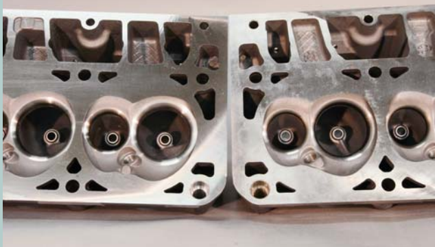
Set side by side, the combustion chambers of the LS7 (left) and L92 show shared features in shape. Valves in the LS7 head, at 2.20 and 1.61 inches respectively, are somewhat larger than in the L92 and won't work on its smaller 4.065 bore (not to mention a 4-inch bore).
