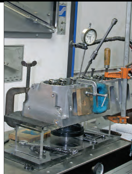
> McKenzie Cylinder Heads, a leading Southern California cylinder-head porter, flowed the LQ9 and L92 heads on its Super-Flow bench. Not surprisingly, the biggest jump was on the intake side, with the new port flowing over 30 percent better at 0.600-inch lift.
