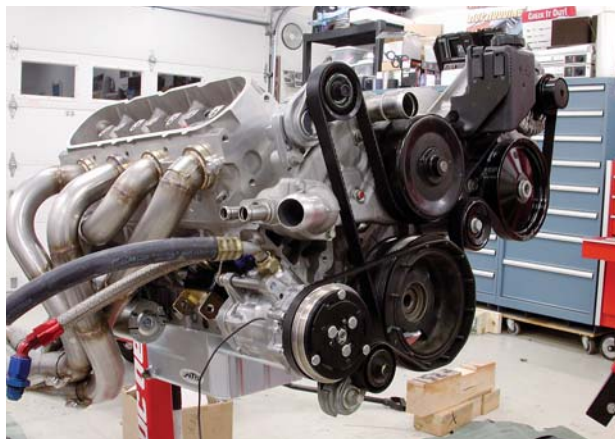
> The accessory drive is a C5 or C6 Corvette assembly with a Vintage Air air-conditioning compressor (PN 04670MTA) spaced forward to clear the stock crossmember.
