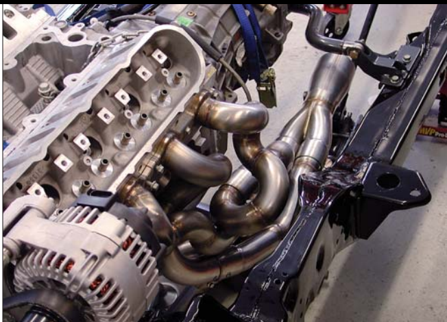
> The ATS tri-Y headers are built out of 304 stainless steel to work with the LS engine mounts in a first-gen F-body. At $1,999, they're pricey, but the tri-Y design really helps the ground clearance, and the headers fit the stock subframe great.
