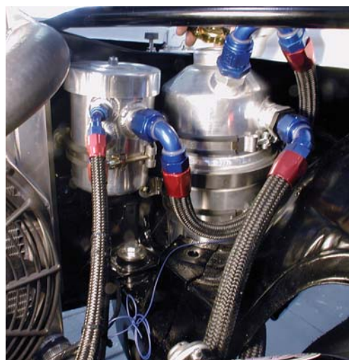
> Below: The other parts of the dry-sump system are the tank (right) and breather (left). The best-fitting oil tank is a Peterson 2-gallon tank (PN 08-0005) with a -12AN pickup, a -12AN return, and a -12AN breather. The oil pump is behind the engine's harmonic damper.
