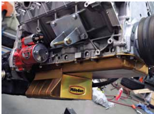
> Here's the second half of the Muscle Rods mount as seen bolted to the engine. Also note our MSD starter and Milodon oil pan. A stock F-car oil pan would have fit in the truck, but we already had the Milodon kit installed on the engine.
