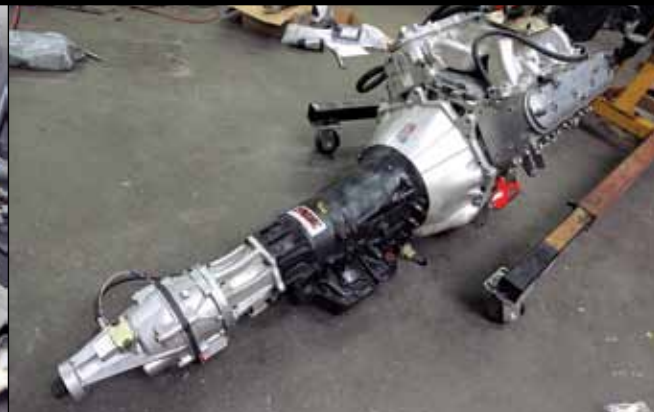
> Here's our lengthy drivetrain, including the GM Performance Parts LS6 crate engine [PN 17801268] that can be had for $5,300 via mail order. We mated it to a Dynamic Racing Transmissions TH400 that has an SFI-approved UltraBell bellhousing from JW Performance. The Gear Vendors Under/Overdrive offers an extra gear of 0.78:1 that can be activated in any transmission gear, turning the three-speed into a six-speed.
