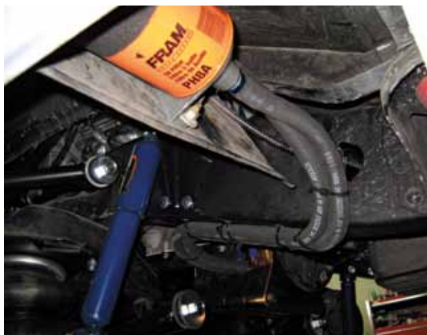
> The Milodon rear-sump pan uses a billet plate to align with the oil feed holes in the block and feed oil to a remote filter. The pan also comes with the hoses and spin-on filter adapter. We located the filter on the backside of the front left fenderwell.
