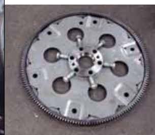
> The distance from the bellhousing surface to the crank flange is different on a Gen III engine than it is on an old Chevy V-8, so this spacer and bolt package is required to hook the conventional trans to the newer engine. These are all GM parts: PN 2551367 for the flexplate, 12563532 for the spacer, and 12563533 [you'll need a quantity of six] for the bolts.
