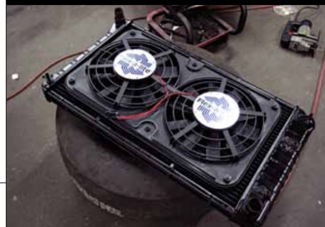
> Since the LS6 does not accept a mechanical fan, we used Flex-a-lite's PN 210 unit with dual 12-inch fans. The 26 1/4 x 15 1/2-inch fan combo fit perfectly on the stock radiator, which we had recored.
