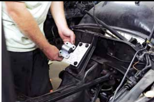
> We used a conversion kit from Muscle Rods to mate the Gen III LS6 engine to the truck. The stock setup uses clamshell-style engine mounts that get thrown away. The stock frame mounts are then redrilled, using the provided template, to install the BRP spool-type mount. The kit was fantastic, but knowing what we know now, we would have scooted the engine rearward an extra inch.
