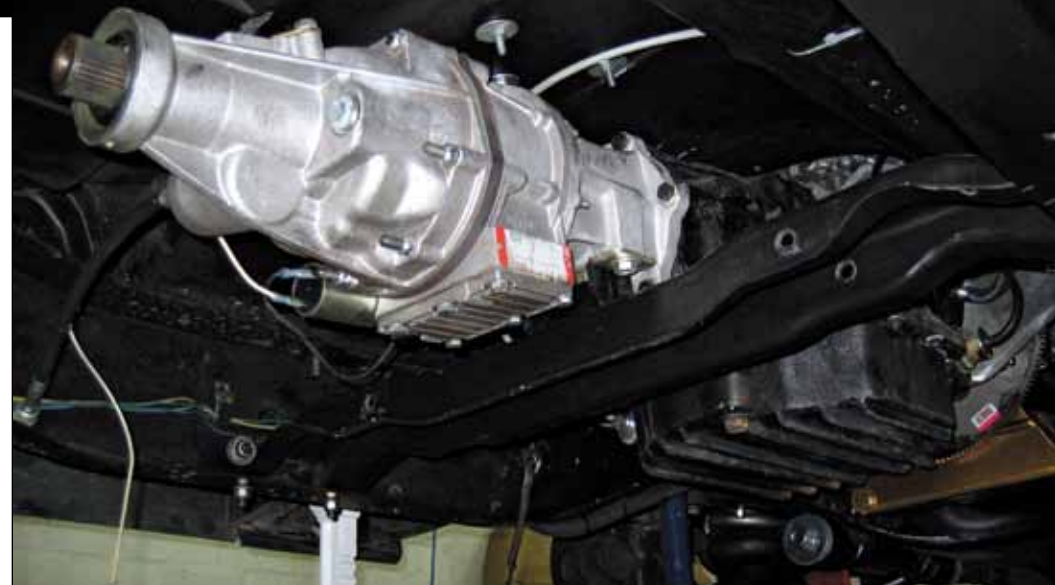
> With the new drivetrain installed in the truck, it was an easy deal to slide the stock trans crossmember rearward on the frame to line up with the mount on the Gear Vendors, then drill new holes to secure the crossmember. The extra length of the GV requires a new driveshaft, but we needed one for our custom engine location, lowered suspension, and Ford 9-inch rearend, anyway.
