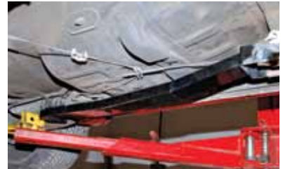
> Designed to follow the body structure without cutting into or interfering with the floorpan, the Hotchkis connectors are formed from 1.5x3.0-inch, 0.120-wall rectangular steel tubing. While it sure is pretty, the brand-new powdercoating must be ground off to obtain sound welds.
