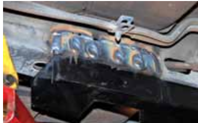
> The Hotchkis connectors are designed for weld-in installation, though the front mount can be bolted in place to allow future subframe removal if desired. On the E-Rod, rosette and circumference welds were laid in with the MIG rig at both ends of the connectors for maximum strength.
