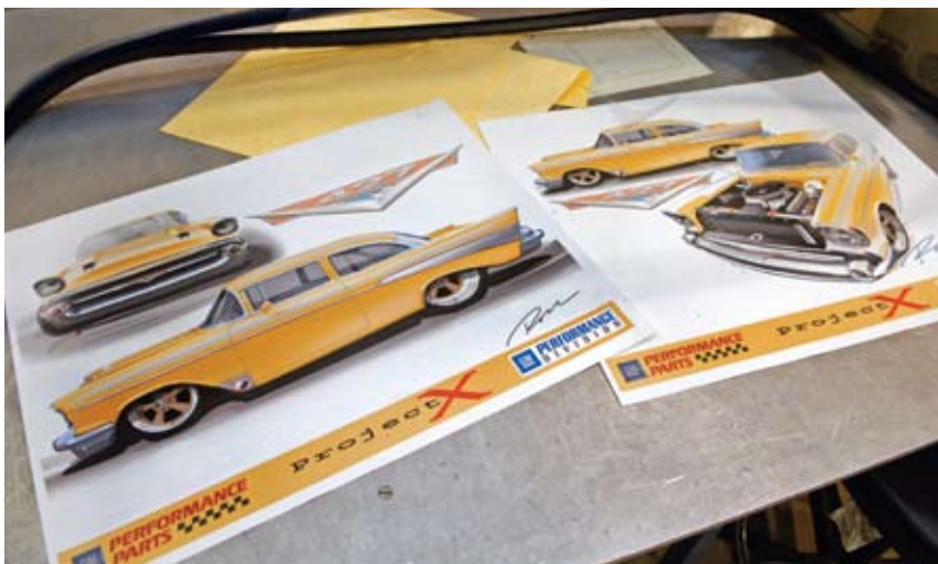
Project X may look the same to some, but GM has designed a lot of subtle upgrades for the car. Side exhaust, a killer retro rim design, a lowered stance with full tire travel, and a functional ram air hood only hint at the work ahead.
