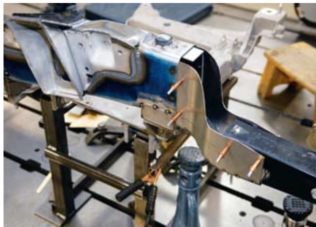
Here's the forward section of the framerrail. The Corvette frame is taller, and therefore had to step down to the '57 frame in the front so the bumper could be bolted to the car.
