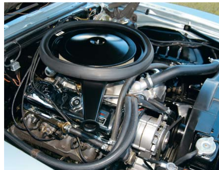
At roughly 500 lbs, the ZL1 was significantly lighter than the L88, weighing about the same as the L46 small-block. The Camaro ZL1 used a single snorkel air cleaner with an open element and gasket that snugged up to the underside of the ZL2 cowl induction hood.
