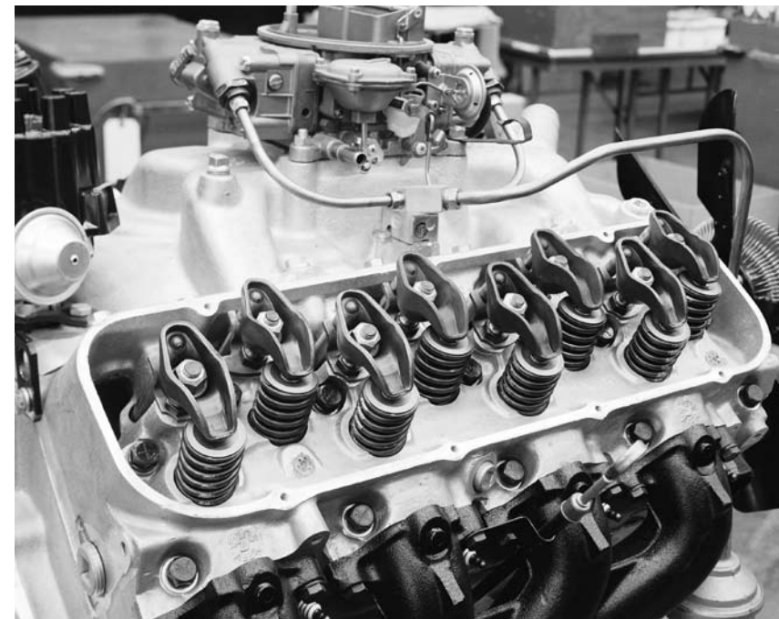
Here's a 1969 427 ZL1. The valvetrain featured 1.70 rockers and specific inner and outer valvesprings for the ZL1. The dual-plane aluminum intake manifold was topped by an 850-cfm Holley four-barrel double pumper with mechanical secondaries.
