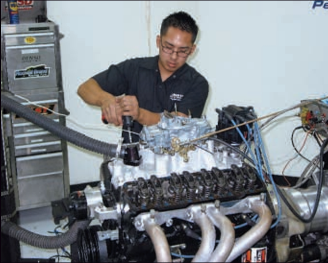
Once the baselines were completed, Eugene (one of the talented Westech dyno technicians on staff) began swapping out the stock stamped rockers.
