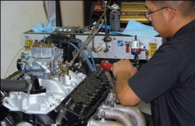
The components should be in near-new condition since we're working on a fresh engine, but an inspection of the pushrods, rocker arm studs, and stud bosses is always a good idea. You should always closely inspect these items if you're performing a rocker arm swap on a used engine; in fact, it's best to swap out the original pushrods for new ones when changing rockers so all components have a fresh start and break in together.
