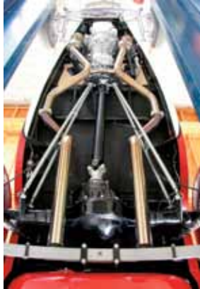
View from underneath the roadster shows the exhaust system minus mufflers, making for an uncluttered and spacious under-carriage.
