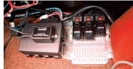
Supplied GMPP LS3 engine wiring harness and engine control module were mounted under the dash against the firewall. It can be mounted in the engine compartment but keep away from excessive heat (exhaust) or in an area that may be exposed to splash from driving in wet conditions.
