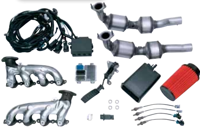
GMPP LS3 engine wiring harness, engine control module, exhaust manifolds, catalytic converters, oxygen sensors and sensor bosses, fuel tank evaporative emissions canister, mass airflow sensor and sensor boss, accelerator pedal (fly-by-wire LS3's electronic throttle), air filter, and instruction manual (not shown).
