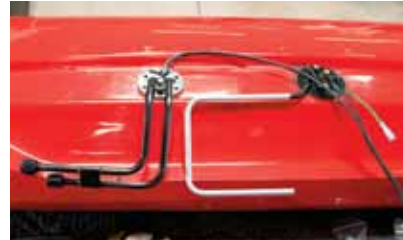
The original '32 gas tank was retained; note the fuel tank evaporative emissions canister line (silver in color, center of photo) needs to be adapted to the tank as it is a vital component to the emission system.
