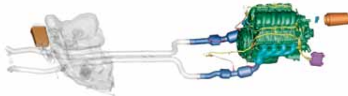
The drawing shows the relative position of all E-ROD components as it might be found in a new Camaro SS.
