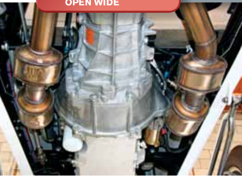
Underneath looking up you can see the four converters in position "wrapping" the six-speed box; plenty of clearance.
