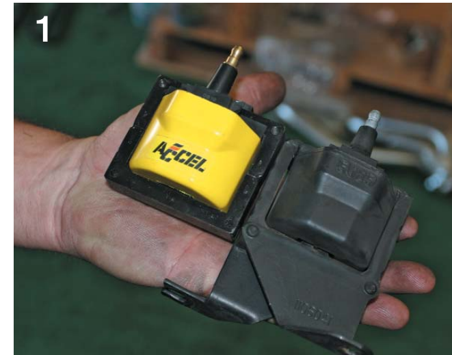
1 For increased throttle response, idle quality and starting we upgraded to an Accel GM HEI remote mount 1984-95 super coil. This coil supplies up to 48,000 volts and will increase idle quality and keep up with the spark demands of our small-block beast.
