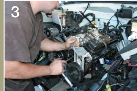
2 Marcel installs the GMPP brackets and pulleys along with the new GMPP alternator. GM Performance Parts makes installation easy with clearly labeled hardware.
