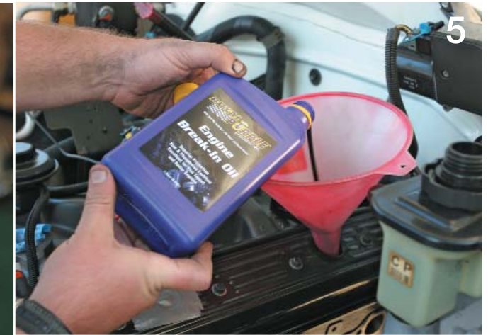
5 For proper break-in we used Royal Purple Engine Break-in Oil. This Royal Purple product is designed for optimum ring seal and to protect rotating assemblies from initial start up wear. Formulated from refined mineral oil and joined with high levels of zinc and phosphorus, the Royal Purple Break-In Oil is the perfect diet for young flat tappet and roller engines.
