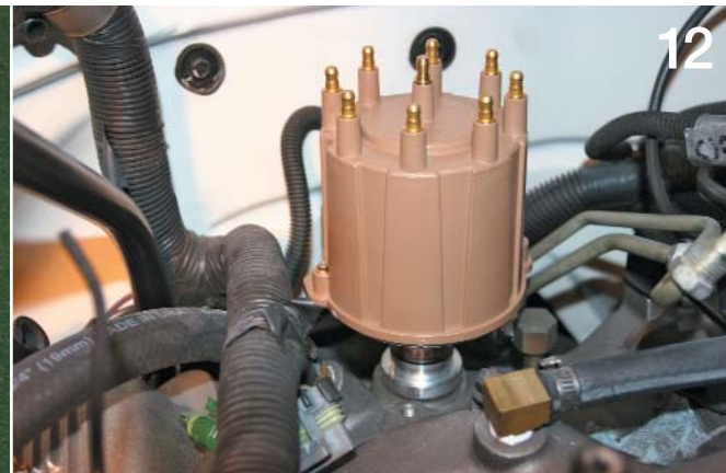
The Accel BilleTech distributor is in place and once we run wires will be ready to ignite our throaty 383.
