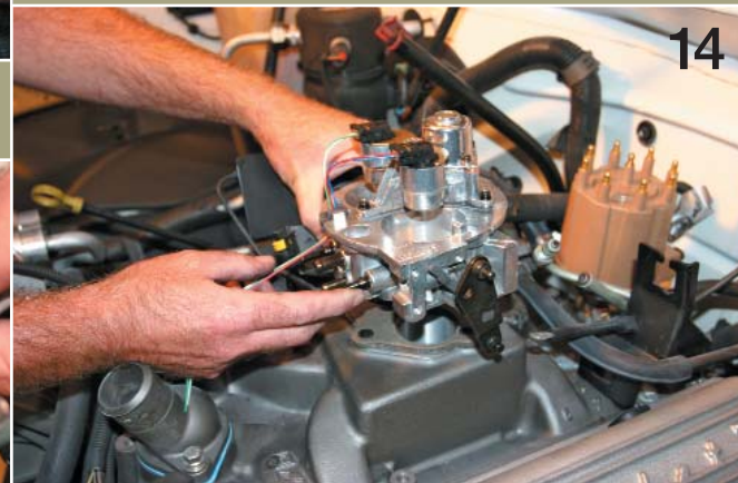
For better fuel delivery and top end performance we installed this Holley Performance Products replacement throttle body obtained from the well-stocked shelves at Summit Racing Equipment. Holley claims a 25 percent increase in torque and horsepower on a stock 5.7L V-8. The replacement TBI is a 670-CFM two-barrel unit and should deliver the perfect amount of fuel to our tire-frying 383.
