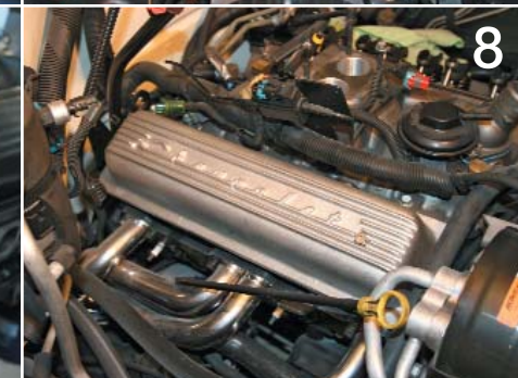
6 From the start of this project the goal was to create a muscle car era look on the sheet metal, under the hood and between the doors. With that in mind we called up the folks at PML for a set of their sand cast, finned and Chevrolet script valve covers. The vintage Corvette look of these valve covers is right at home on our GMPP 383 and fit the theme perfectly. They utilize the two outside holes on a center bolt head for mounting.
