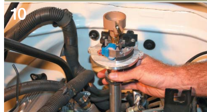
The distributor is slid into the back of the manifold and lined up with the cam gear.
