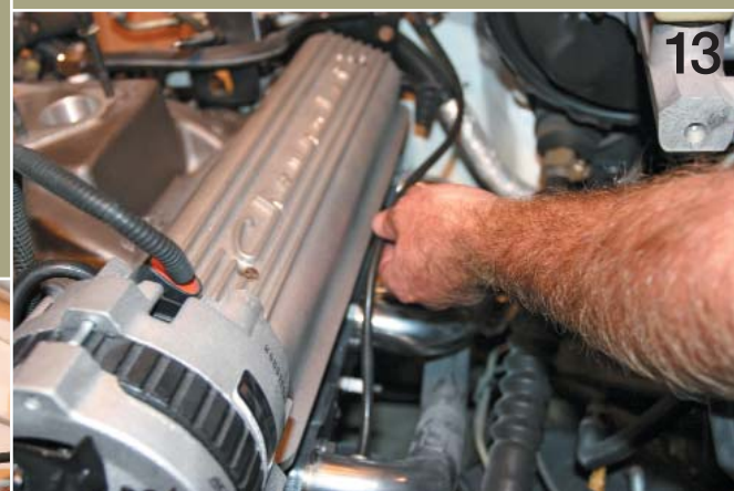
Mike runs the Accel Extreme 9000 wires to the candles. These wires feature ceramic boots and are rated to withstand 2,000° F. They should hold up well next to our Gibson tubes.
