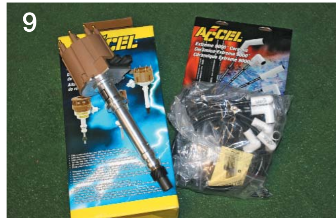
To upgrade our small-block's spark path we dropped in a fresh BilleTech distributor from Accel. All Accel BilleTech distributors feature a 6061 T6 billet aluminum housing, center-less ground steel shaft, 10,000-RPM bearing upper with oil lite bushing lower, and Accel performance electronic pick up and module. Topped by a high dielectric strength cap and balanced rotor, the BilleTech distributor is a recipe for trouble-free performance. Brass cap contacts and an iron or steel distributor gear compatible with flat tap-pet cams and OEM hydraulic roller camshafts finish off this performance distributor. Accel Extreme 9000 wires were also thrown into the mix for supreme durability, especially when run right next to scorching hot headers.
