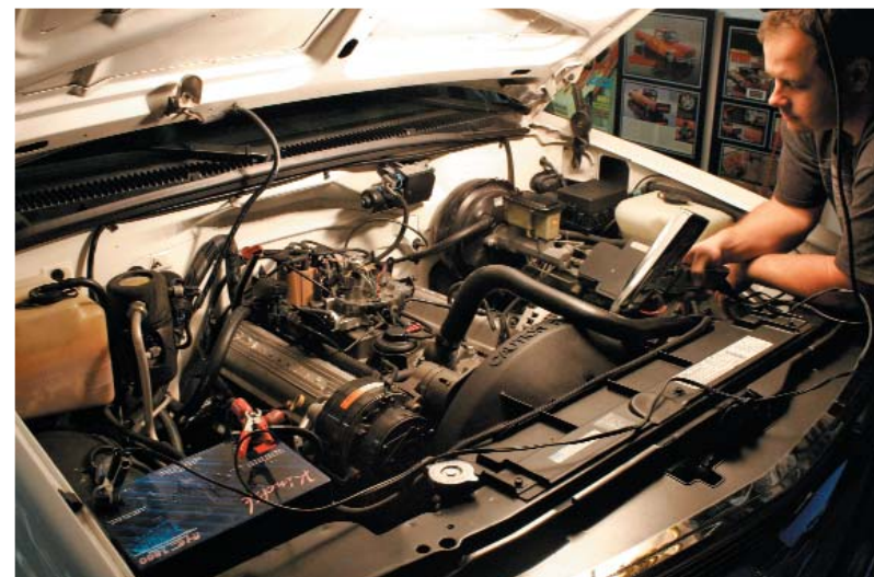
We followed GM Performance Parts' recommended timing specifications, fired the torque monster 383, and held the gun steady while the 383 gave us its sweet spot.
