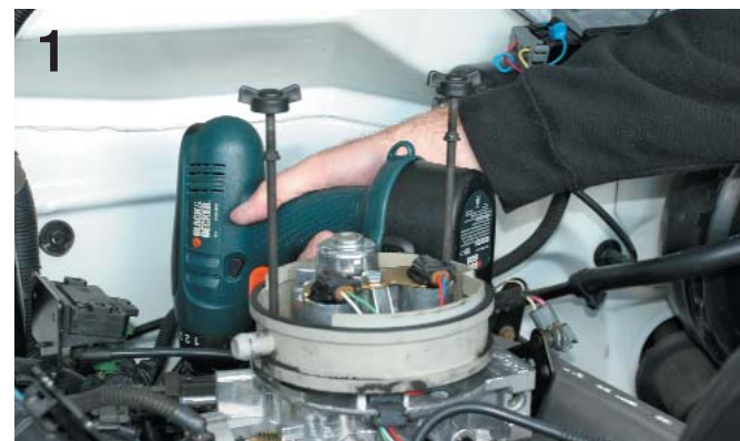
1 Before our 383 spoke its first words, and since we had not yet set the timing, we took a few minutes to pull the distributor and hook our oil primer to a drill motor and spin the oil pump. This will get oil cycled throughout the motor and prevent the lifter valley from running dry when we crank the key for the first time.
