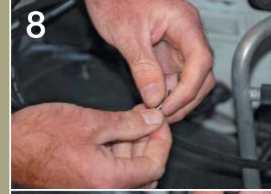
8 The end of the wire terminal is crimped into place and the boot is slipped over the wire. These wires from Accel are called the Extreme 9000 and are designed to take extreme temperatures without burning and causing misfires.
