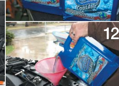
11 To keep our new 383 cool we poured in Be Cool Coolant, which is rated for 300,000 miles and is premixed and ready to use. We replaced the radiator after the new engine went in because the original one was filled with corrosion. With a brand-new engine you don't want to take any chances. Next month, we will melt the rear tires off this truck and give you our view from the driver's seat.
