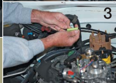
2 Mike marked the wires and began tracing them to the appropriate candles. Take your time going off the firing order on the intake manifold.
