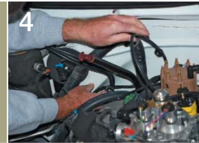
4 The Accel Extreme 9000 wires are snaked down nice and clean, and Mike calculates the length to each spark plug before snipping the wire and crimping on the boots.
