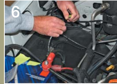
5 Using a razor blade, Mike trims the plug wire to the proper length and prepares to strip the end of the wire for application of the plug boot.
