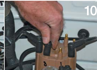
10 Each wire is run from the distributor to corresponding spark plug per the firing order indicated on the intake manifold. Mike takes his time to run each wire one at a time, being careful not to cross any wires. Labeling the cap is a smart idea to prevent mixing anything up.
