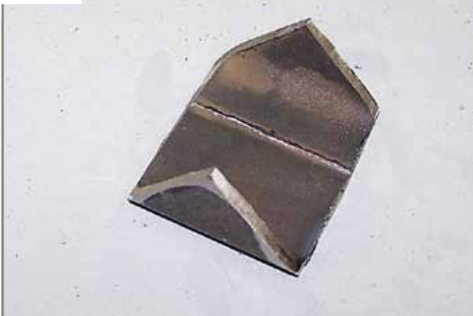
Side pieces were fabricated to be welded in place on the crossmember. Pieces were MIG welded in place, and then ground smooth.
