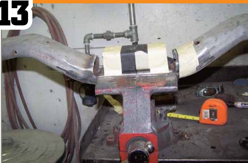
Our 4L80E application called for a modified crossmember, so a chunk was removed from the center section. The lower mounting point for the transmission would create more room in the trans tunnel. A reinforcement plate is cut to size to serve as the base for the transmission mount.
