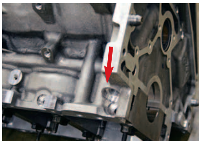
A look at the rear corner of the LS7 block shows the inlet for the engine's dry-sump oiling system.
